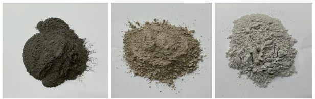
(a)粉煤灰 (b)脱硫石膏 (c)矿渣 图 1 粉煤灰、矿粉和脱硫石膏的实物图
